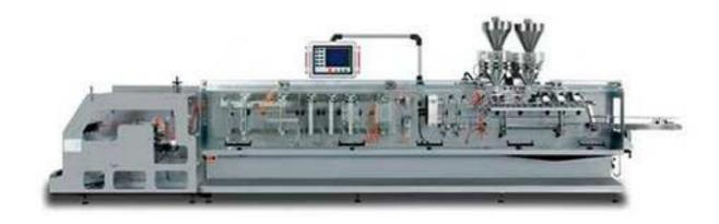
SC-180 Series designed for doypack, with functions of making hanging hole, special shape, Zipper or spout.
