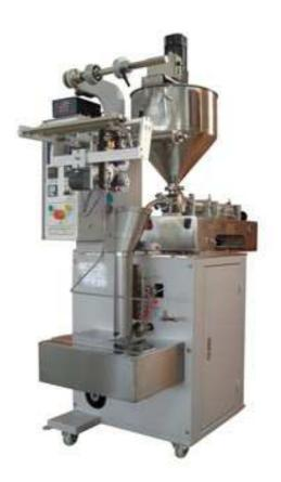
The machine adopts a series of more function bag-making in three sides cutting packaging machine. According to different measuring system, it is to extend packaging granular, liquid, sauce, powder machine features. It is suitable 30-300ml products automatic packaging.
