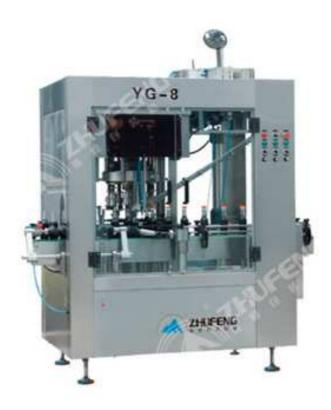
This machine is rotary lid-presser, (after change can also have press inner plug function), mainly use for sealing of foodstuff, such as soy sauce, vinegar, cooking wine, cooking oil and daily chemical products and other non-threaded plastic caps. This machine has 8 capping head, can automatically arrange caps, drop caps, catch caps, capping and out bottles. The machine operation convenient, stable performance, production speed fast, high pass rate, has good sealing performance after capping.
