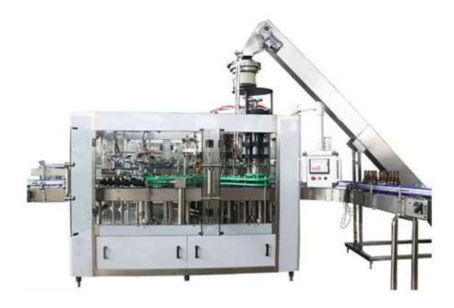
Our newly designed BCGF serious monoblack beer filling machine is designed for bottle filling, it can suit for PET bottle and glass bottle size between 150ml to 2000ml, can customized to maximum of 3000ml. Genus design of capping design makes different screw cap change into one simple easy torch. On machine surface is only leaving 3 points of bearing support point which makes drainage so easy and without any dirt stain.
