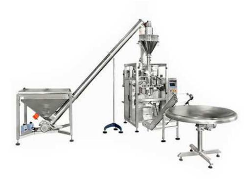
Powder packing machine is mainly for spice powder, coffee powder, milk powder etc into small bags, by matching with weigher, or liquid pump.
