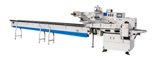
The machine model FFE is applicable for the packaging of biscuit with multi rows and columns, multi-bag vitellus pie, French bread, snowy biscuit, and other kinds of bulk products with family or group packing. The machine makes the package available for the biscuit with family&group packing automatically, takes the place of manual packing, with advanced technology in the domestic and international market.
