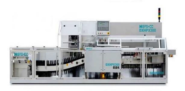
Auto high speed Cartoning machine, up to 300 cartons/min
