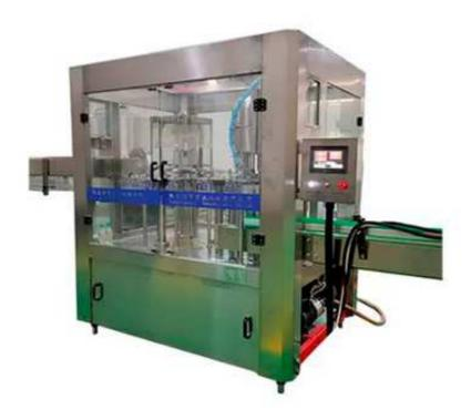
Automatic mineral water bottle 3-in-1 filling monoblock, combined with rinsing, filling and capping. It is innovated and designed in the requirement of still pure water and mineral water, on the bases of introducing, digesting and absorbing advanced technology from Germany and Italy.
