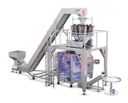
The latest German technology has been used to manufacture this industrial line, such as the compressed air systems, drive and control sensors, and optical sensors, in order to provide good performance, high speed and continuity of work for 24/7. It is equipped for the purpose of packing the (all Kind of Chips and Nuts, legumes, beans, rice).
