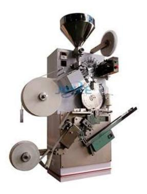
This is our high speed automatic tea packing machine, it makes filter tea bag with cotton thread and tag, the speed 110 bags/min. There is auto boxing device, vacuum feeding device, heat sealing tag device, stirrer, date printing machine optional.
