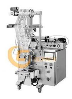
The machine can be equipped with date coding device, nitrogen gas filling device, easy tear device, punching device, gusset device ect.
