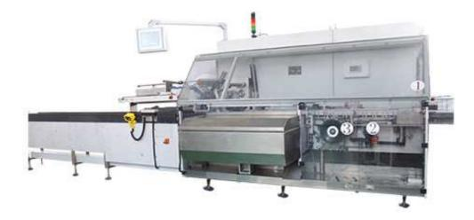
HZJ200 Cartoner is mainly used for toothpaste and pharmaceutical. It is designed with hot glue sealing or tucker type sealing systems. The control parts are of international famous brand and with Chinese / English touch screen, which is very convenient to operate.
