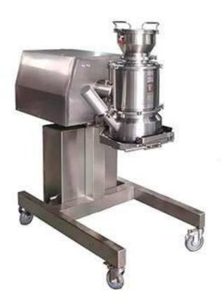
Cone milling is one of the most common methods of milling in the pharmaceutical, food, cosmetics, fine chemical and associated industries. They are typically used for size reduction and deagglomeration or delumping of powders and granules.
