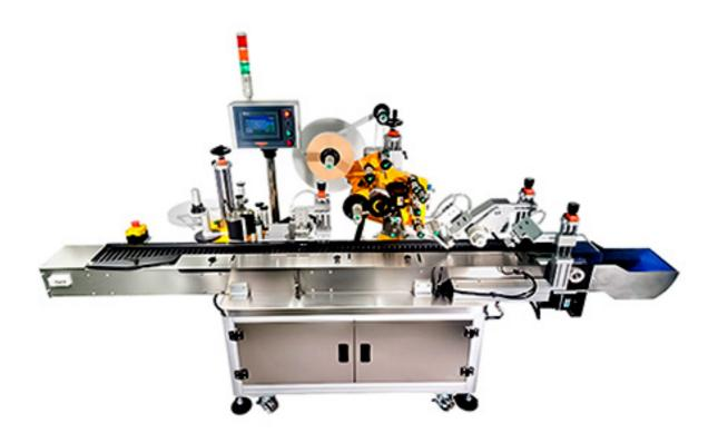
Suitable for precise labeling on the surface of various cylinder containers which is applied to the bottom of pen-shaped containers (lipstick, lip gloss, mascara) in the cosmetic industry labeling.
