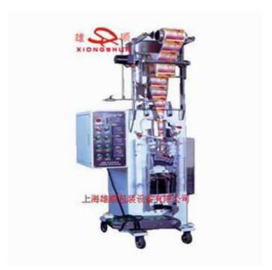
This series machines are same to DXDY60/B machine of packing, making sack filling, sealing and counting. The different is the cutting off number of bags can be changed by setting.
