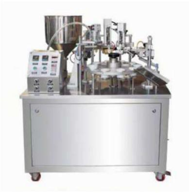
DTG250 series tube filling and sealing machine is used for both plastic tubes or laminated tubes. The technology used is cam system and copper heating to finish the tube feeding, eye-mark, automatic filling, tube heating, code printing, tail trimming and automatic ejection. It is widely used pharmacy, cosmetics, and chemical, adhesive and food industries.
