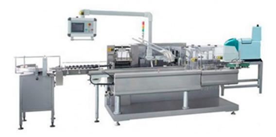
DZH-120 automatic cartoning machine can be applied to various products including bottles of perfume, cosmetics, eye drops, etc. together with extra functions such as cartoning, leaflet folding, code printing, carton closing and sealing, etc. PLC control system is applied for which the machine is able to shut down automatic upon errors. The machine can be used individually as well as be connected to other types of machine.
