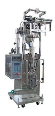
The process of measuring, bag-making, filling, sealing, printing and cutting can be done automatically.
