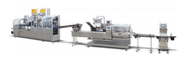
The packaging line can be widely used for packing different size of capsule, tablet and solid products (Alu-PVC/Alu-Alu) blister packing and cartoning. Can be connected with weighing machine, strapping machine, carton packer and other equipment, thus formed a complete automatic packaging production line.
