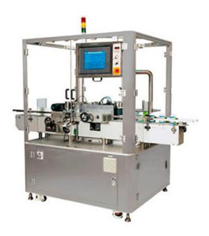
Multipack machinery provides automatic vertical linear sticker labeling machine model MULTIPACK-60F which is one of the most user friendly. It is used for applying label on front, back or side for oval/flat/square/round/ shape containers with labelling speed of up to 100 labels per minute depending upon products size/shape and label size. It is synchronized with top holding belt system.
