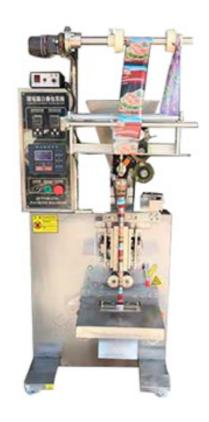
This automatic chili powder sachet packing machine can automatically complete bag making, measuring, filling, inflating, counting, sealing, code printing, material giving, stopping in certain quantity, fixed-bag cutting and same cutting, with CE Certification. The spice masala packing machine can be used to pack different kinds of powder.
