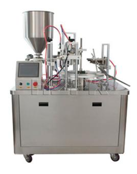
This machine is a high technical equipment, it is an ideal equipment for plastic tubes and multiple tubes filling and sealing in cosmetic, pharmacy, foodstuff, adhesives etc industries.
