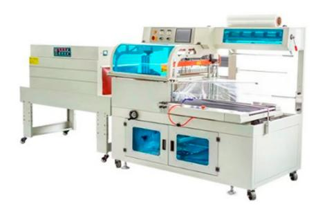
Automatic L-Bar Sealer is an entry-level automatic sealer which provides an economical, durable and easy-operated solution for packaging. It is also widely applicable to various industries such as toys, cosmetics, tools foods, stationeries, daily commodities, electric appliances, etc. With the uniqueness of the perforation system, it has been successfully granted us a leading position in the industry.
