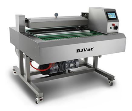
Automatic continuous type vacuum packaging machine continuously operates through the cylinder drive the rotation of the conveyor belt and applies to the product packaging of large productive enterprises. Depending on the different sizes of the contents, one or two sealers could be set within one vacuum chamber in order to improve the working efficiency. The workbench angle could be adjusted according to the features of the contents.
