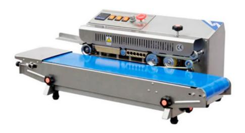
One of our most popular band sealers with a great value propositions. Can seal 20-26 6" wide poly bags per minute. FR-770I is a compact horizontal belt sealer with modern design. On this clever table model pre-made bags are sealed lying flat. All operating parameters are controlled by a digital control panel, including an automatic cool down function.
