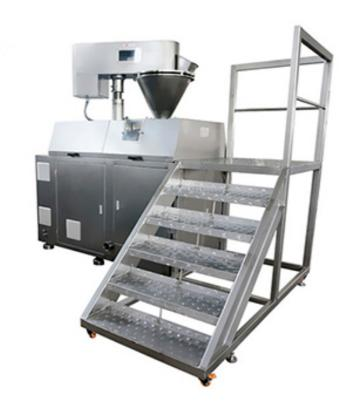
By using the crystallization water in the materials, the equipment can form the granules directly by the condensed water of raw material.
