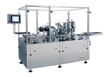
DSG2-A type is an eye drop liquid filling machine our company has developed for the production of ophthalmic medicine. It adopts peristaltic pump and 2 head fixed filling.
