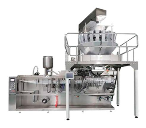
BHS-210D is specially designed for small and medium-sized flat bags, and can produce two bags at a time, doubling the production capacity. The packaging capacity is 150ml. Three-side sealing or four-side sealing can be selected according to customer needs, or the shape of the edge sealing. It is often used to package cosmetics, insecticide powder, medicines, etc.
