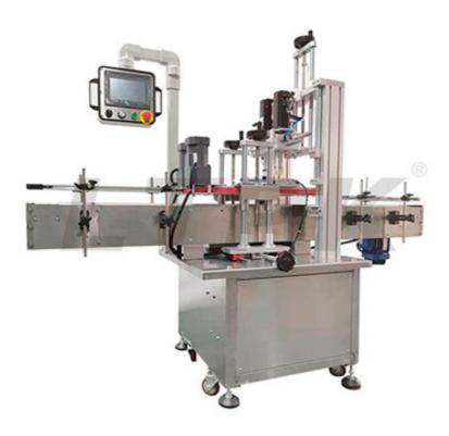
This machine is used for capping closures for bottles or jars. It uses robotic arms for screwing, which is easy to adjust and suitable for many kinds of screw caps, such as flat screw caps and sprayer screw caps. It is widely used in the drinks, daily chemical, and biological industries.
