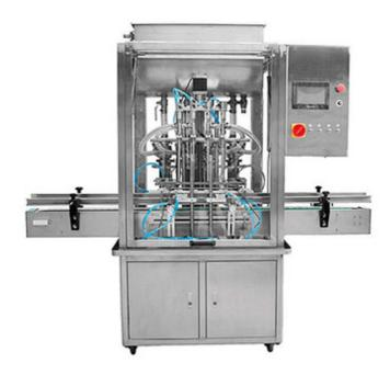
Piston fillers are a great option for packaging liquids. They offer fast and accurate fill rates, versatility with the ability to handle many different types of products, and they're gentle on products. They're ideal for viscous liquids including batters, sauces, pastes, icing, chunky fillings, and certain aerated products. Generally, these liquid packing machines are used to fill liquids that are squeezed through pastry bags or similar packaging.
