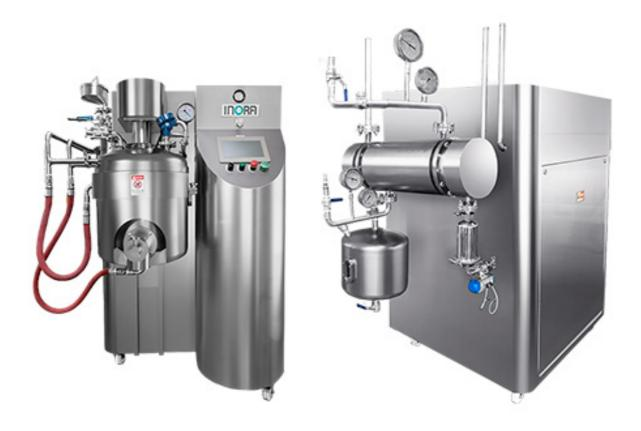
Inside the cone-shaped vessel, the main impeller mix the powder into fluidized vortex and form lumps with the cinder solution. Then the high speed chopper cut the lumps into even granules by high speed action.
