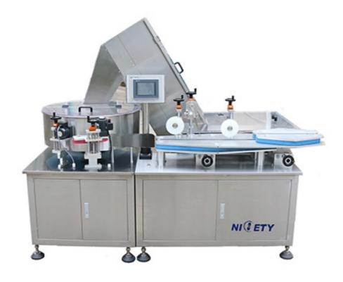
Pour the bottles into the buffer hopper and the machine sort the bottles in upwards position and automatically transmitted to conveyor orderly.
