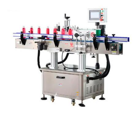
The machine can simultaneously achieve two-sided circumferential surface labeling and labeling features to satisfy the flat bottles, square bottles and bottle shaped single-sided and double side labeling, the entire circumference of the cylindrical body a half weeks labeling, widely used cosmetics industry, daily chemical industry. Optional Tape printer and inkjet printer to achieve the production date printed on the label and batch information to achieve labeling – endowed integration.
