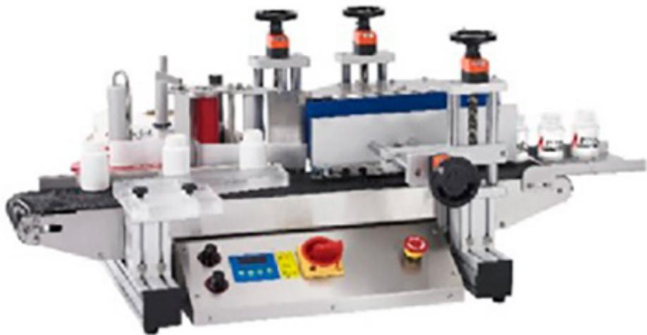
The ALR1100 is a tabletop automatic round bottle labeling machine for various sizes. Supports 360° wrap labeling, 2/3 wrap, half-wrap, and dual-side labeling. Compatible with PE, PET, PP bottles, glass, and metal containers. Provides precise, smooth label application to enhance product appearance. Features an intuitive microcomputer control system for easy operation, ideal for small-scale production, cosmetics labeling, food & beverage labeling, and pharmaceutical bottle labeling.
