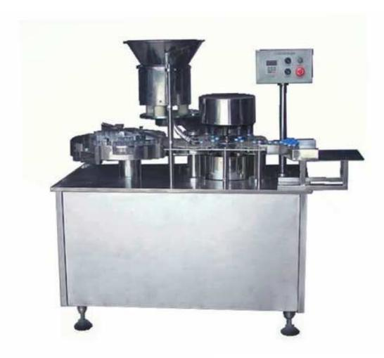
This machine is applicable to an aluminum cover for small dripping bottle and clinical bottle to seal, use six heads roll a side, pressure size to adjust the convenience, and replace the bottle specification to only need to replace to adjust a little amount spare parts. This machine the frame is simple, and the adaptability is strong.
