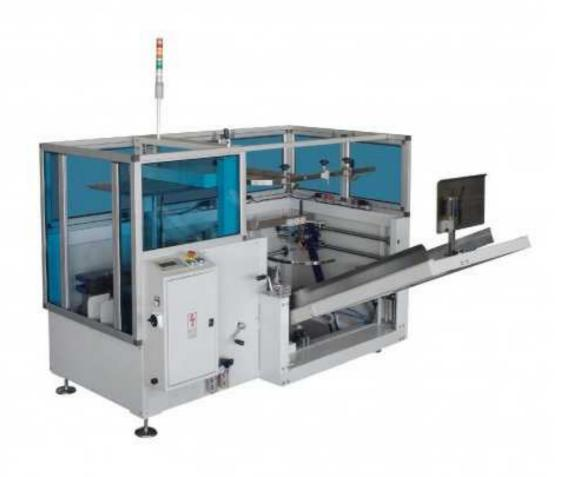
Case erectors and case cartoners are case equipment which automatically forms corrugated cases. A stack of corrugated blanks are knocked down and placed into the machine. The blanks are pulled out of the machine one-by-one and formed into cases. The newly formed cases are sealed at the bottom with tape or glue.
