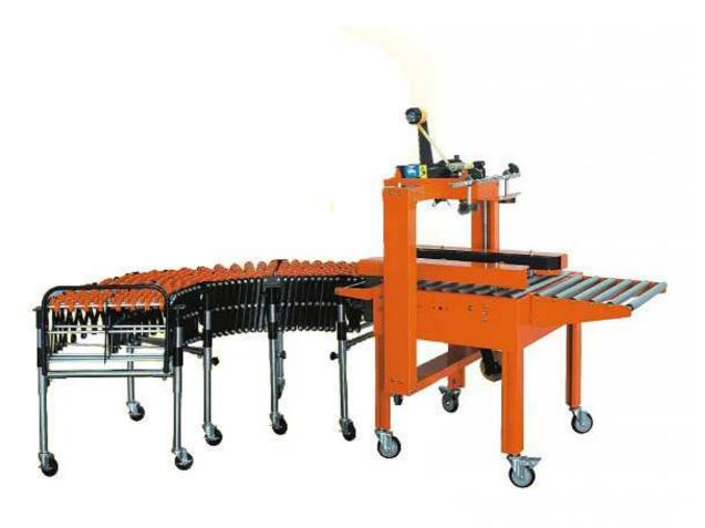
Carton sealers are case equipment that seals the top or bottom of a case with tape or glue. Typically, the minor corrugated flaps are kicked and plowed closed as the cases are transferred. As the cases enter the compression section, the major flaps of the carton are closed and a hotmelt adhesive is applied.
