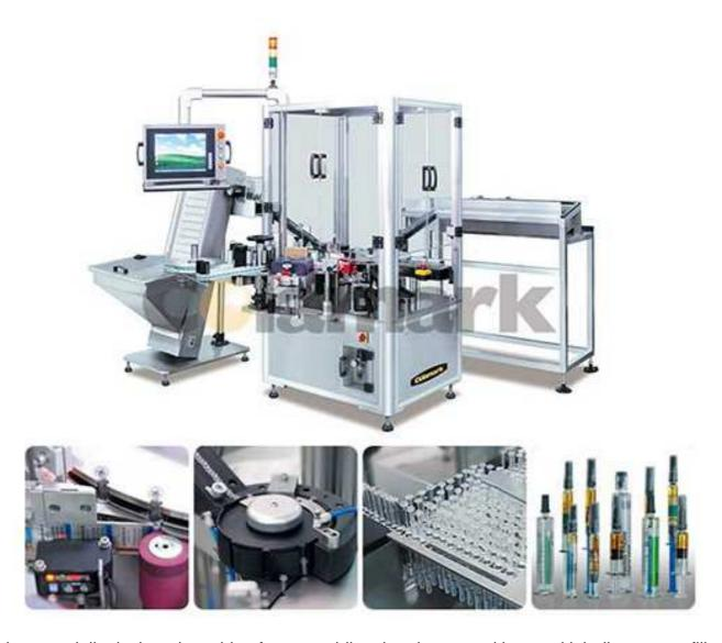
A11 is a specially designed machine for assembling the plunger-rod into and labeling on pre-filled syringes.
