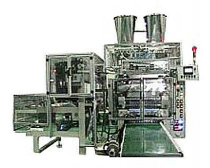
This Model AP-1200P can attain the maximum speed up to 60 SPM that helps to do speedily packaging of powder and granules. This model with its electronic web edge controlled mechanism is perfect for packing and sealing approx. 300 grams of product. Its 4 side sealing offers absolute safety and helps to efficiently seal free flow powder & granules products.
