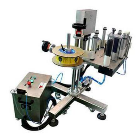
Online labeling applicator, can be related to the production line, the flow of products, on the plane, curved labeling, implementing online marking, realize supporting to spurt the code conveyor belt, the flow through the object labeling
