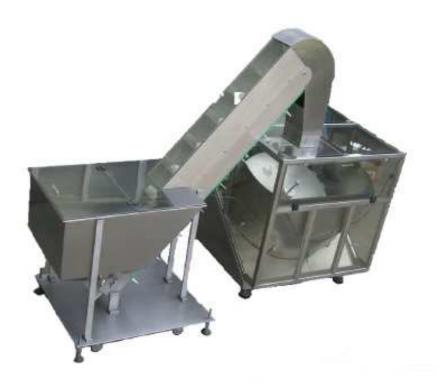
SLP-1800 can sort round bottles automatically and put the containers stand on conveyor with high speed – 150 BPM. The unscrambler consists of main sorting unit, cover with door, bottle feeding elevator and storage tank. It is easy to operate and stable running and widely used in the pharmacy, food & beverage, cosmetic & personal care industries.
