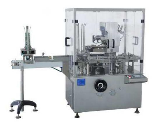
DZ-120B Blister Card Cartoning Machine Suitable for automatic cartoning and box sealing of aluminum-plastic / aluminum-plastic-aluminum / aluminum-aluminum medicine plates, pillow type packing bags, oral liquid trays, suppositories, plasters, facial masks, eye masks, etc. in medicine, food, health products, cosmetics and other industries.
