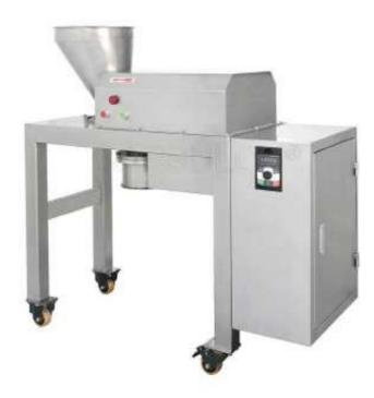
This machine is used mainly in such trades as pharmacy, chemical industry, food, pottery, and plastics extensively, making moist powder material particle. Make cylinder swing reciprocally, extruding material from screen mesh for granulation. It also can be used for crushing the agglomerate materials into small granules directly.
