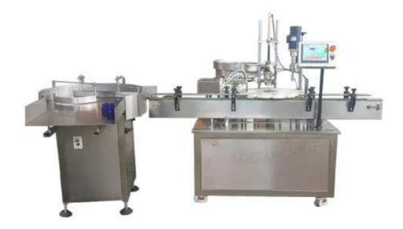
This machine is mainly available to fill small bottle into various round and flat plastic bottles or glass bottle with the range from 10-150ml. High precision cam provides a regular plate to position, cork and cap; accelerating cam makes capping heads going up and down; constant turning arm screws caps; peristaltic pump measures filling volume; and touch screen controls all action.
