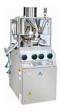
Tab Xpress-PTX Tablet Press Machine is used for production of simple and precise tablets from powder in Pharmaceutical and relevant Industries.
