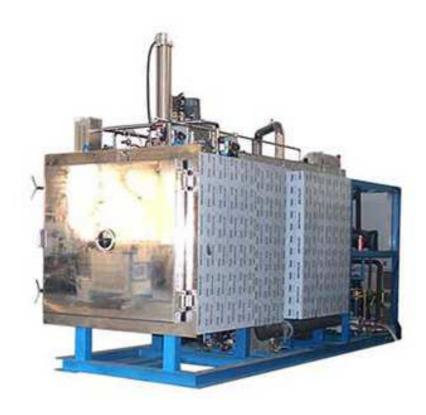
Freeze-drying is widely used in the pharmaceutical industry to stabilize drug products. During lyophilization, solvent is removed from solid phase (direct sublimation, or gas phase) to produce a dry product that can be readily reconstituted to its original liquid formulation by the addition of solvent. The process extend shelf life of the product by inhibiting chemical and physical degradation pathways that occur in the presence of moisture.
