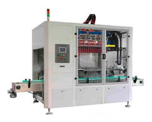
This type machine is design according product, and the clamp is designed for the different products. Clamp clamped by products, automatic positioning in the carton, when the fixture is raised, automatic discharge, finished product packing. it also apply to similar product packing bottle shape. The characteristics of the machine is multi-usage, is suitable for a variety of specifications products, fixture replacement simple easy to operate, convenient adjustment, industry widely.
