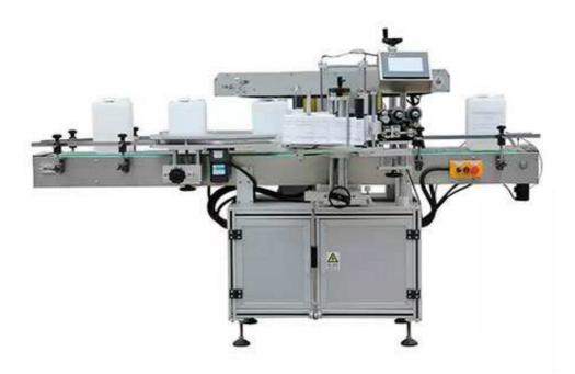
The production line is mainly used for single and double side sticker labeling. After a round bottle matching device. Can simultaneously solve the self-adhesive labeling round bottle surface.
