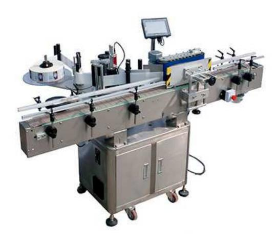
This kind of Automatic Adhesive Labeling Machine is suitable for flat bottle to label control system adopted Panasonic Stepper two-axis PLC control, collocation large LCD human interface, it is easily to operate, servo motor control label. This machine is made of SUS304 and aluminum alloy.
