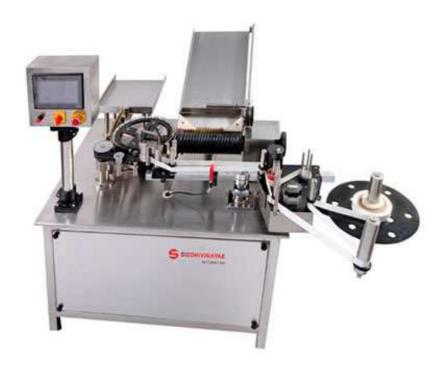
Ampoule Vial Rotary Sticker Labeling Machine - The SVAARL 200/ 300 is a fully automatic vertical rotary sticker labeling machine. This machine is suitable to apply full/partial wrap around self adhesive labels precisely on different size of round ampoule/vial.
